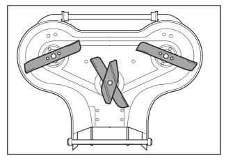
Cutting unit (rear ejection)
